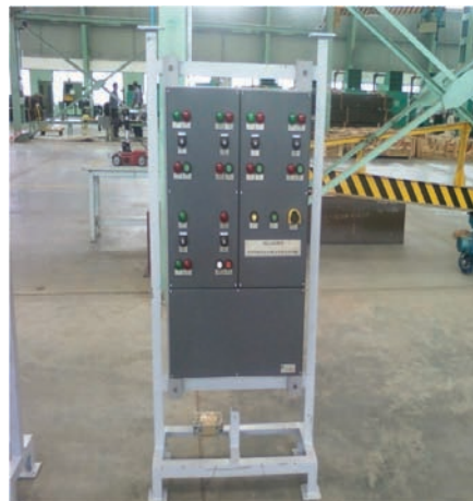
Photo of Micro PLC Based Logic Reduced 40% in size & components
