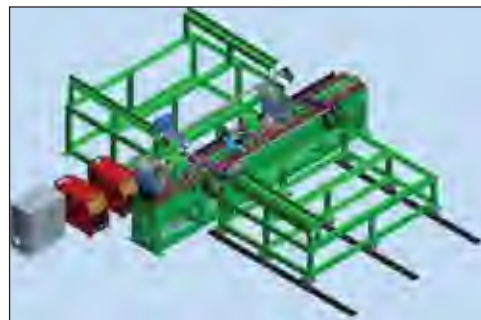
IDLER ROLLER WELDING SYSTEM – FULLY AUTOMATIC WITH LOADING & UNLOADING SYSTEM
