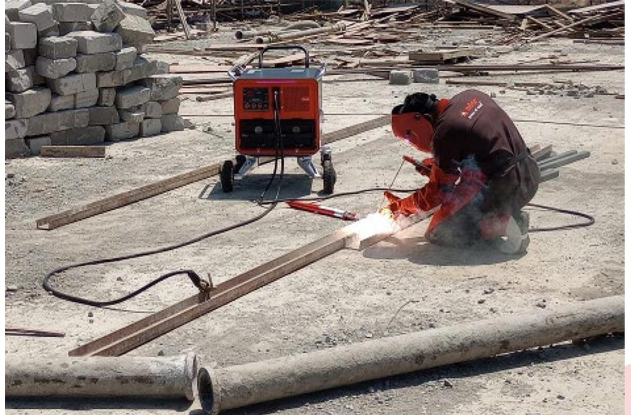
THIS BATTERY POWERED WELDING MACHINE IS BEING USED ALONG WITH ARC SENSING MIG/ MAG WIRE FEEDER IN EUROPE FOR RAILWAY TRACK MAINTENANCE
